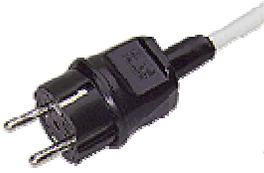
The 'Schuko' plug is moulded together with the power cord. To re-wire, cut off the moulded plug from the power cord. It is advised that this be replaced by appropriately rated mains plug such as 13AMP or 15AMP mains plug.
