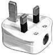
**The 13AMP 3 pin fused Mains Plug** – This is used for electrical appliances such as refrigerators, washing machines and microwave ovens. As these appliances have metal body, the body must be grounded so that in the event of electricity leakage to the metal body, there is no risk of electrocution to human.
